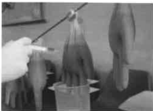
Fig Washing of the external surface of the glove with double distilled water
