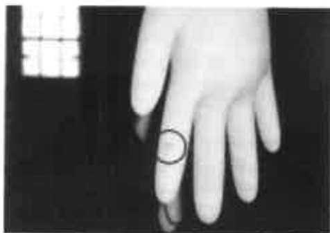
Fig The round circle exhibits site of micro defect
